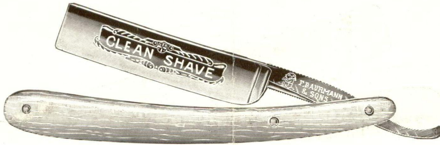
No. 462.— \frac{5}{8} " wide full hollow ground, hollow blue polished, tang and back crocus polished, file tang, etched in silver round ivory celluloid handles with stop.
